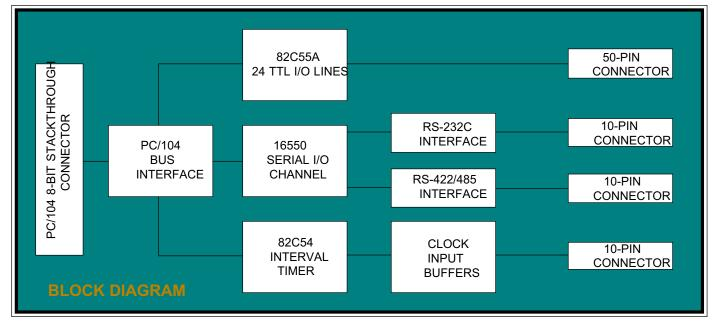
and C. Ports A and B are programmable as 8-bit groups of input or output lines. Port C is programmable as two 4-bit groups of input or output lines. Provisions for implementing an interrupt driven strobed I/O mode are also included using option jumpers. A 10K pull-up resistor is connected to each I/O line for accommodating input connections. I/O connections are provided by a 50-pin connector that is Opto-22 (or eqivalent) compatible.
